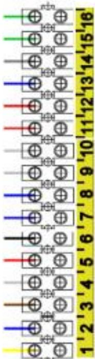
15-16 KESSELFÜHLER (optional NTC 10K) KESSEL THERMOSTAT (optional)
